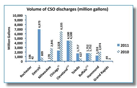
Figure 2. CSO discharge volumes for 2010, 2011. Includes only raw sewage discharge volume (partially treated discharges — those discharges undergoing primary treatment and, in some cases, disinfection — from Detroit were 49,634 million gallons in 2011, and 13,554 million gallons in 2010).
